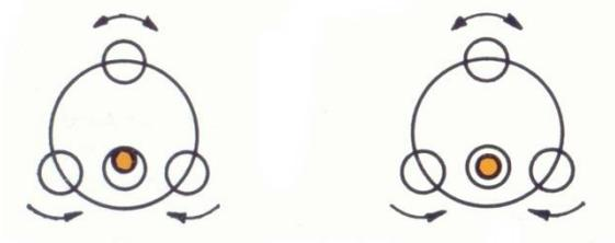
**Instrument is ready for taking readings if bubble is well within etched circles.**
