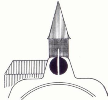
Employ tangent screw [3] to move staff to centre of field of view. By means of focussing knob [7], image is now made to appear sharp.
