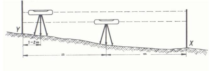
1. At the beginning of this check (possibly with the aid of the tachometric feature of the instrument as described under E), the level is set up exactly in a central position between two levelling staves placed at a distance of about 60 m (choose firm locations for staves, holding them perfectly upright).
