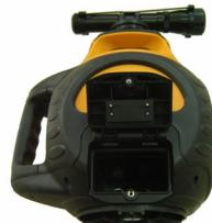
Battery compartment of instrument
