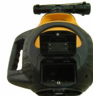
Insert the battery case into the instrument
